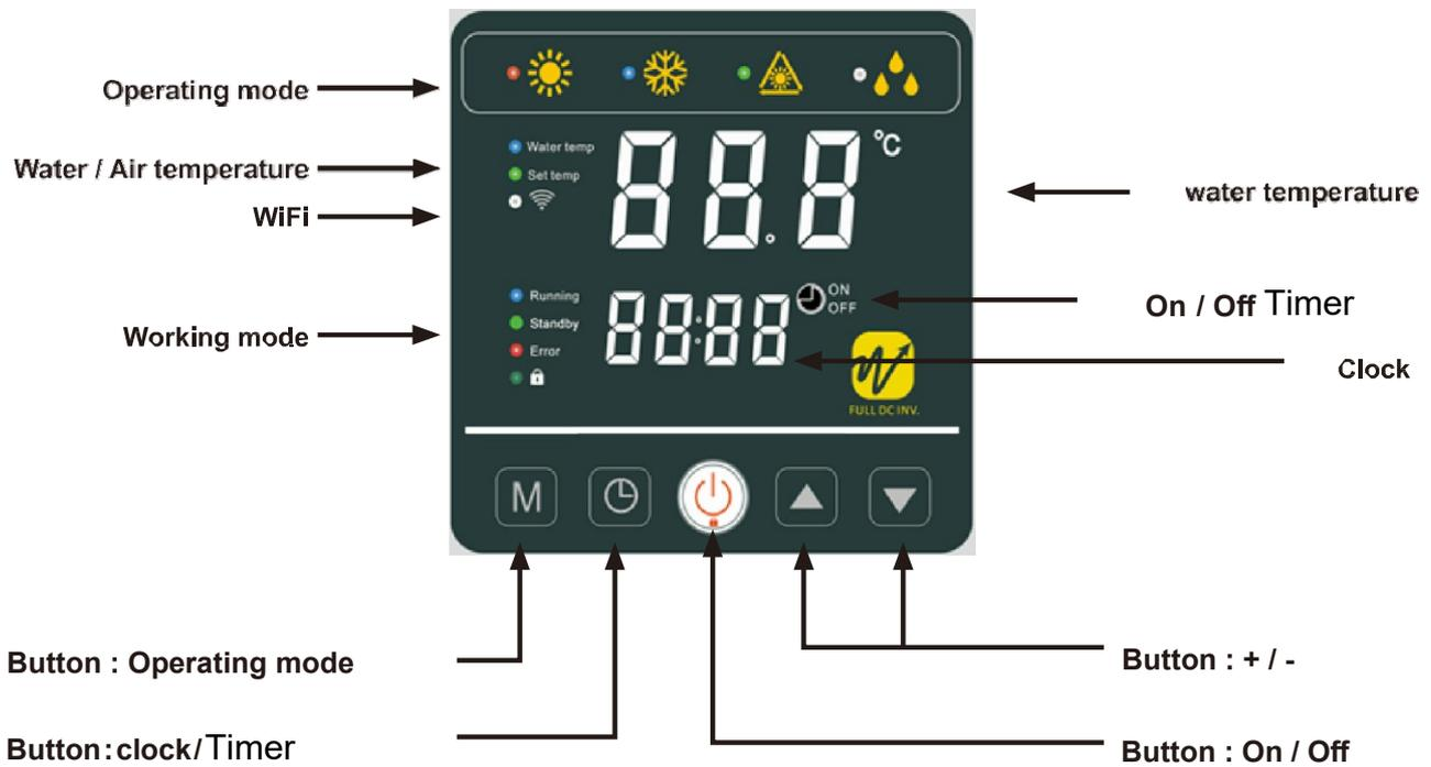
To start the heat pump, press the
