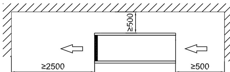
Place nothing less than one metre in front of the heat pump.
