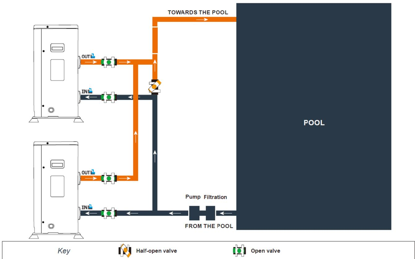
The filter located downstream of the heat pump must be regularly cleared so that the water in the system is clean, thus avoiding the operational problems associated with dirt or clogging in the filter.
